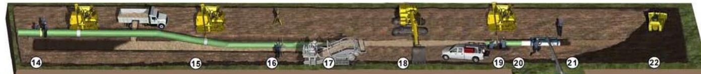
14. Inspect and Repair Coating 15. Lowering-in 16. As-built Survey 17. Pipeline Padding (as needed) 18. Backfill and Preliminary Clean-up 19. Tie-ins 20. Pressure Testing, Final Tie-in 21. Caliper Run and Calibration Digs 22. Clean-up, Restoration, & Seeding/Mulching
