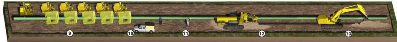
9. Welding 10. Weld, Non-destructive Testing and Repair 11. Coating Field Welds 12. Conventional Trenching: Wheel Ditcher 13. Conventional Trenching: Excavator
