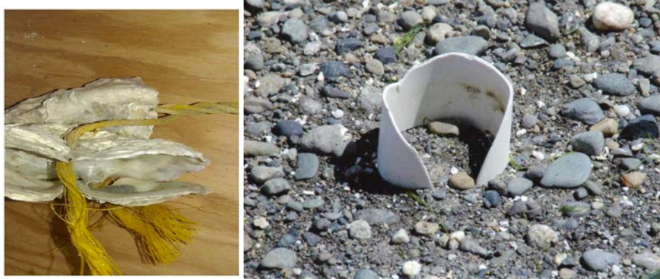
Figure 3 Left: Yellow rope used in long-line culture growing through oyster shell. Right: PVC tube degrading
