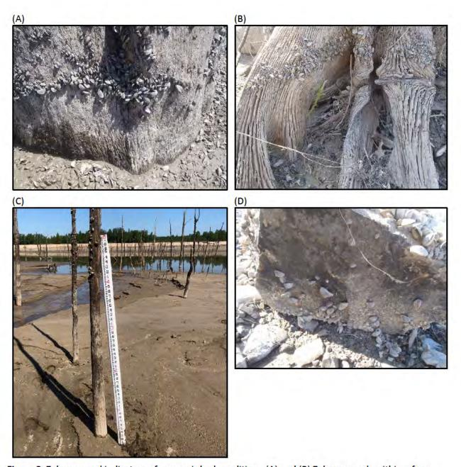
Figure 3 Zebra mussel indicators of reservoir bed condition. (A) and (B) Zebra mussels within a few centimeters of the sediment surface, indicating normal reservoir bed. (C) Zebra mussels about 4 feet above the sediment surface indicating sediment scour, and (D) Zebra mussels on the underside of a large rock, indicating the rock was flipped over by hydraulic conditions during the reservoir drawdown.
