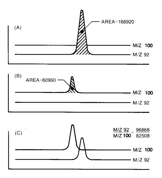
FIGURE 7 Extracted Ion Current Profiles for (A) Toluene, (B) Toluene-dg, and (C) a Mixture of Toluene and Toluene-dg
