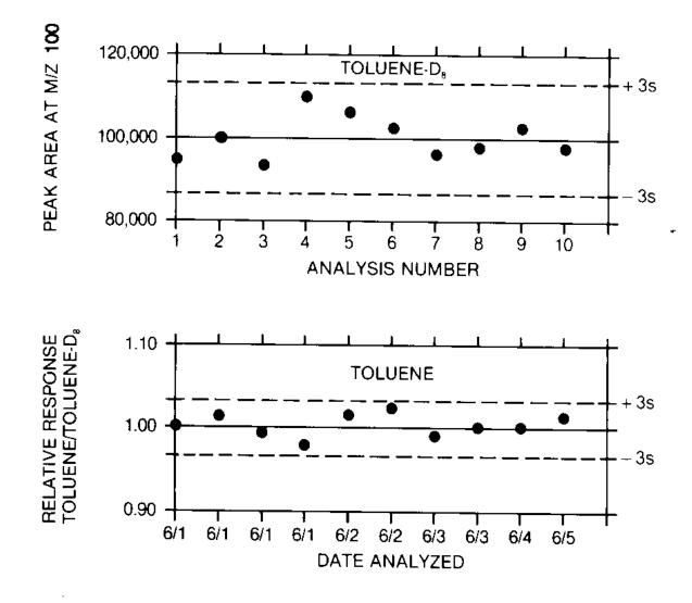
FIGURE 8 Quality Control Charts Showing Area (top graph) and Relative Response of Toluene to Toluene-dg (lower graph) Plotted as Function of Time or Analysis Number
